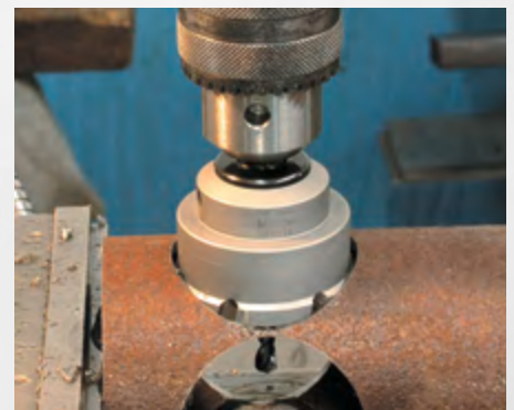
Bohren in Rohre
