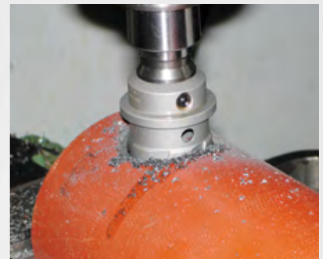
Bohren in Rohre
